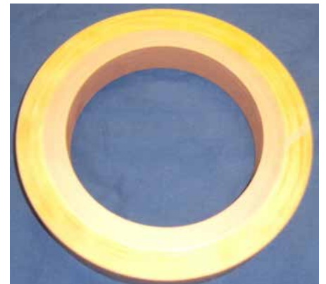
Figure 6. Photograph of a steel ring with 0.05 inch of Cold Spray deposited copper.
