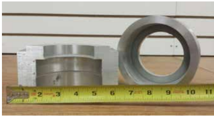
Figure 3. Photograph of the mockup used to develop and validate the Cold Spray repair on the AL-6061 actuator body.
