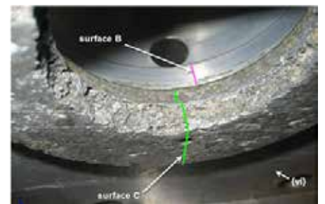
Figure 2. Photograph of the corrosion damage on TD-63.
