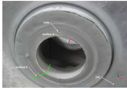
Figure 4. Photograph of the Al-6061 actuator body after Cold Spray deposition.
